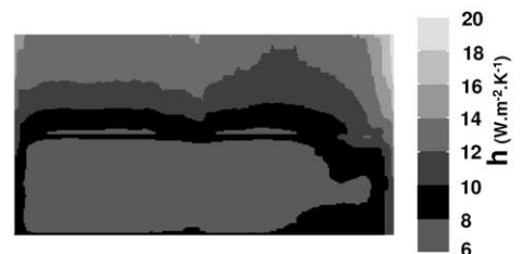
Figure 8. Treatment of the pictures on the side of the cylinder sloped at 45° into the flow: (a) 4 pre-treated initial pictures; (b) example of a temperature profile used to locate the markers; (c) complete image after having pieced together the 4 preceding pictures and corrected the distortions due to the convexity of the surface; (d) image after marker erasing and geometrical resizing.
